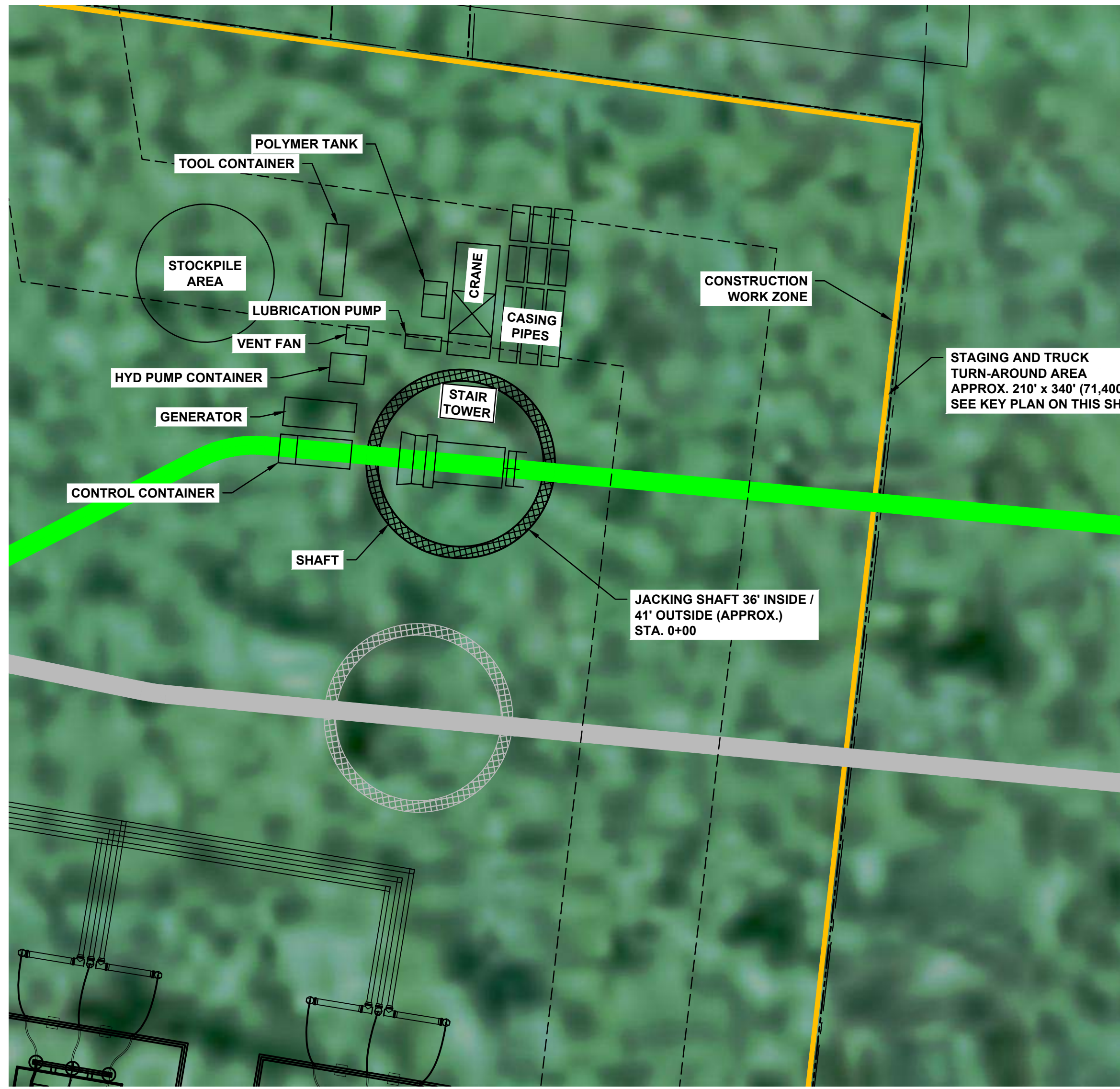
JACKING SHAFT 1 CONSTRUCTION STAGING PLAN 1" = 20'
