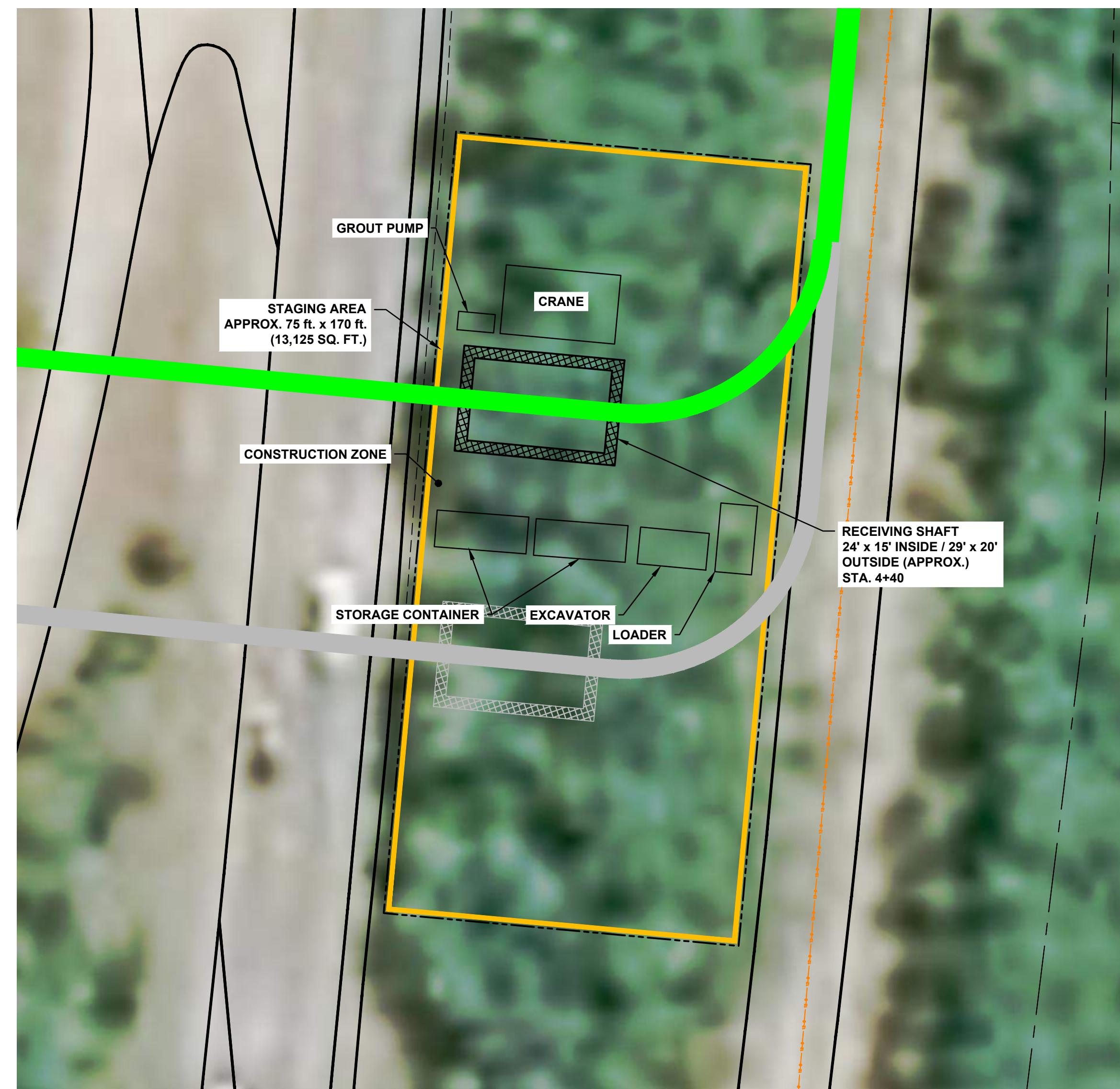
RECEIVING SHAFT 1 CONSTRUCTION STAGING PLAN 1" = 20'
