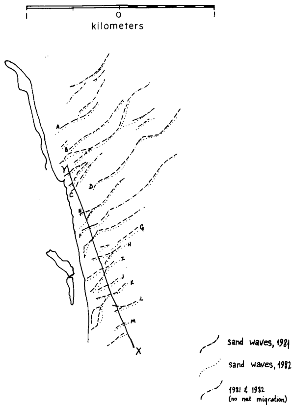
Fig. 4. Sand-wave migration patterns on Popponeset Platform for the period 1981–1982. Location of profile in Fig. 3 is shown.
