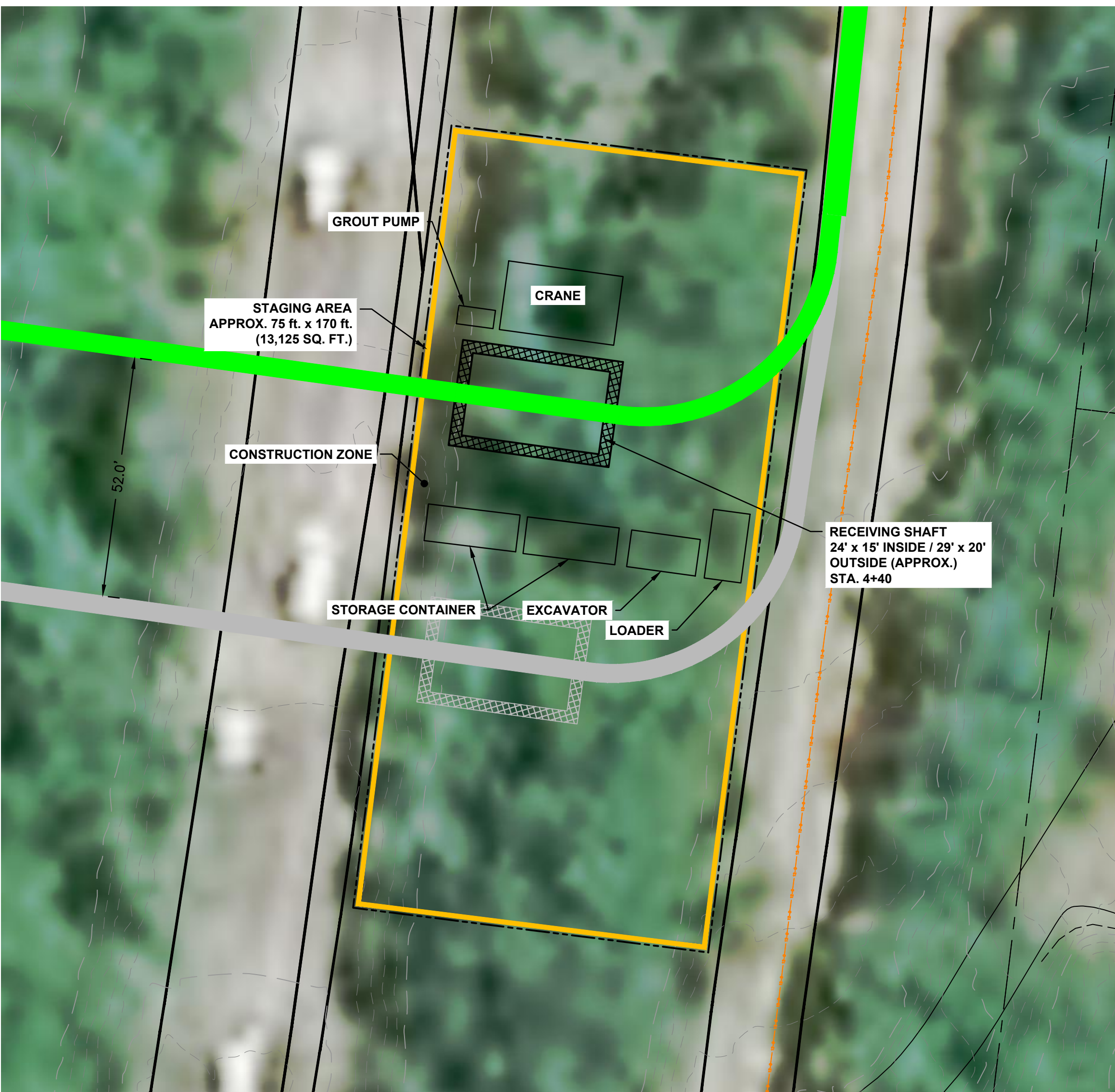
RECEIVING SHAFT 1 CONSTRUCTION STAGING PLAN 1" = 20'
