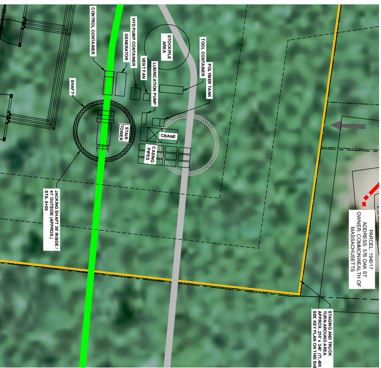
JACKING SHAFT 2 CONSTRUCTION STAGING PLAN 1"=20'
